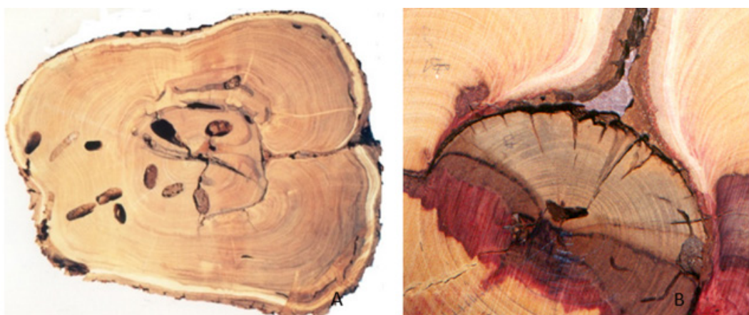
Figure 3: Altered wood by fire scar and insect galleries in Prosopis nigra (Fabaceae) (A). White and brown rots and Fusarium species attack in Aspidosperma quebracho-blanco (Apocynaceae) wood (B).
