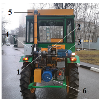
Figure 6: Gas turbine electric generator on a tractor. 1. Gas turbine engine; 2. Three-stage free turbine; 3. Asynchronous electric generator; 4. Switching cabinet for external connections; 5. Air cleaner; 6. Power asynchronous electric motor.
