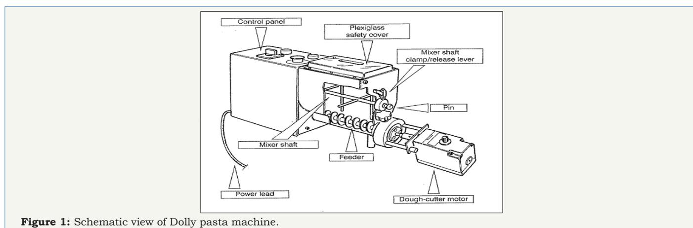
**Figure 1:** Schematic view of Dolly pasta machine.
