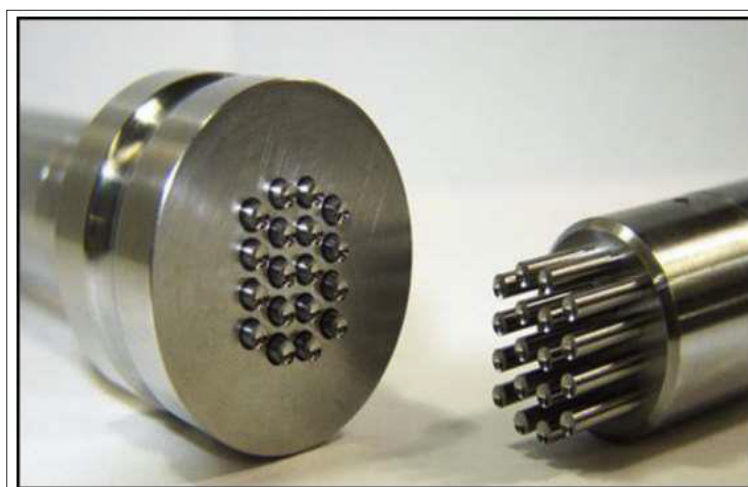
Figure 2: Multi-tip 2mm diameter tooling for manufacture of mini-tablets [1].
