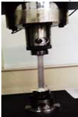
Figure 4: The part mounting and mounting clogs to conduct the compression test.
