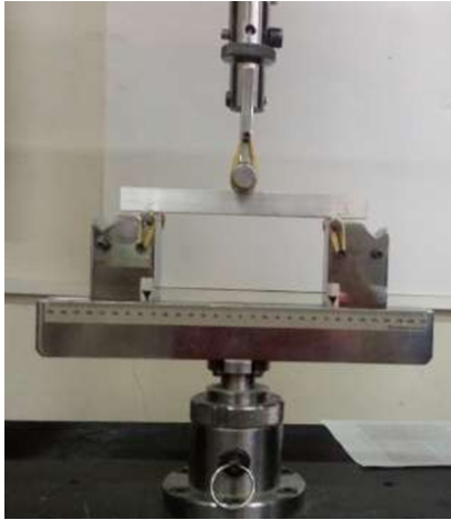
Figure 2: Installation of the part in order to perform the three-points bending test.
