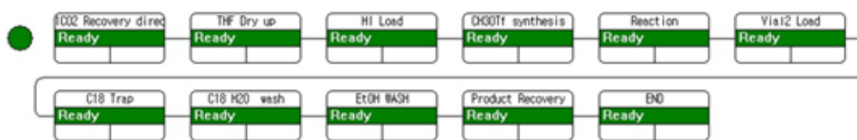
Figure 2: Schematic diagram of the CFN-MPS200 Automated Synthesis Module Program.
