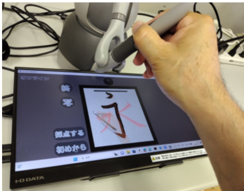
Figure 2: Writing a character using the stylus of the haptic device.
