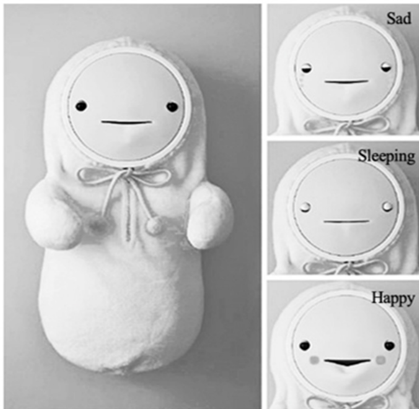
Figure 1: Smibi, the baby robot used in the present study, replicates the reactions of a human baby and is similar in size to a 3-month-old (440mm in height, 200mm in width, 190mm in depth, and 1.2kg in weight).
