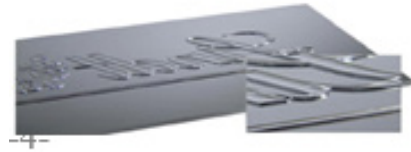
Figure 18: Operation of a positive milling mold.
