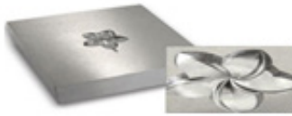
Figure 16: Milling application does not require polishing.
