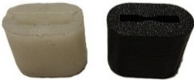
Figure 2: Injection molded neat PP cushion (left), 3D-printed PA6-CF15 cushion (right).
