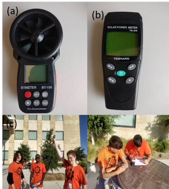
Figure 3: (a) An anemometer; (b) A solar power meter; (c) Students measuring air velocity; and (d) Students measuring solar intensity.
