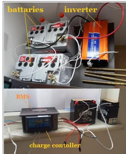
Figure 4: Experimental setup control system with batteries.
