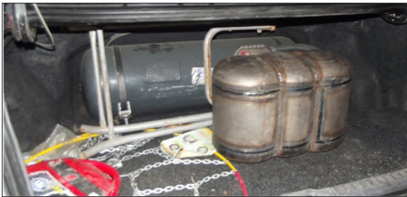
Figure 7: A view of the three-cell 41-liter LPG tank.
