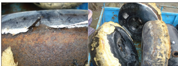
Figure 9: Corroded view of the torus tank mounted on the underside of the vehicle.
