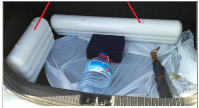
Figure 12: View of the 3 and 4-cell LPG tank with 50% space in the vehicle.
