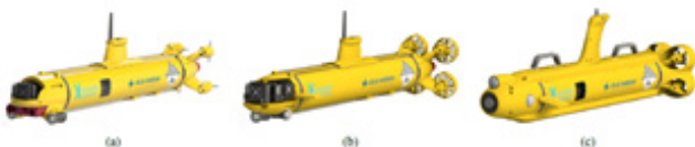
Figure 2: CAD rendering of previous and current version of the AUV. (a) Mk. 1.0, (b) Mk. 1.1, (c) Mk. 1.2.
