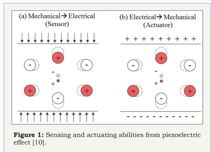
**Figure 1:** Sensing and actuating abilities from piezoelectric effect [10].
