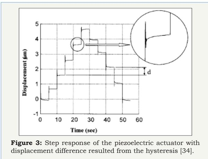
**Figure 3:** Step response of the piezoelectric actuator with displacement difference resulted from the hysteresis [34].
