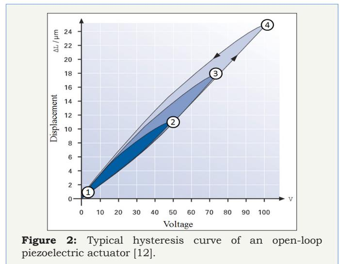
Figure 2: Typical hysteresis curve of an open-loop piezoelectric actuator [12].
