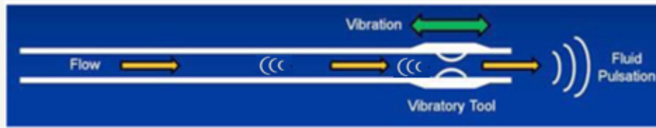
Figure 1: Working mechanism of hydraulic axial vibratory tool [22].
