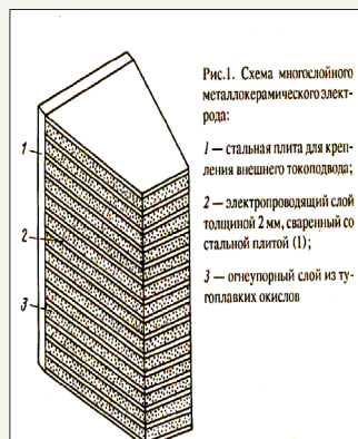
Figure 2: Many-layer metal-ceramic anode: 1-base steel plate for fastening external current wiring; 2-electro conducting steel sheets of thickness 2mm; 3-refractory ceramics.
