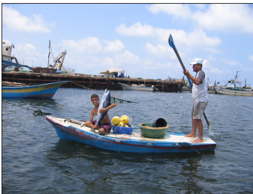
Figure 3: The non-motorized hasaka (oar-drawn hasaka) is the most common fishing boat used by fishermen in the mediterranean ecosystem of the Gaza Strip.
