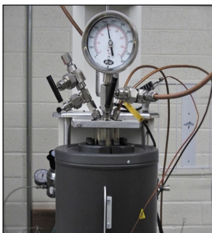
Figure 2: 500-mL HTL pressure reactor used to transform halotolerant microalgae into biocrude.
