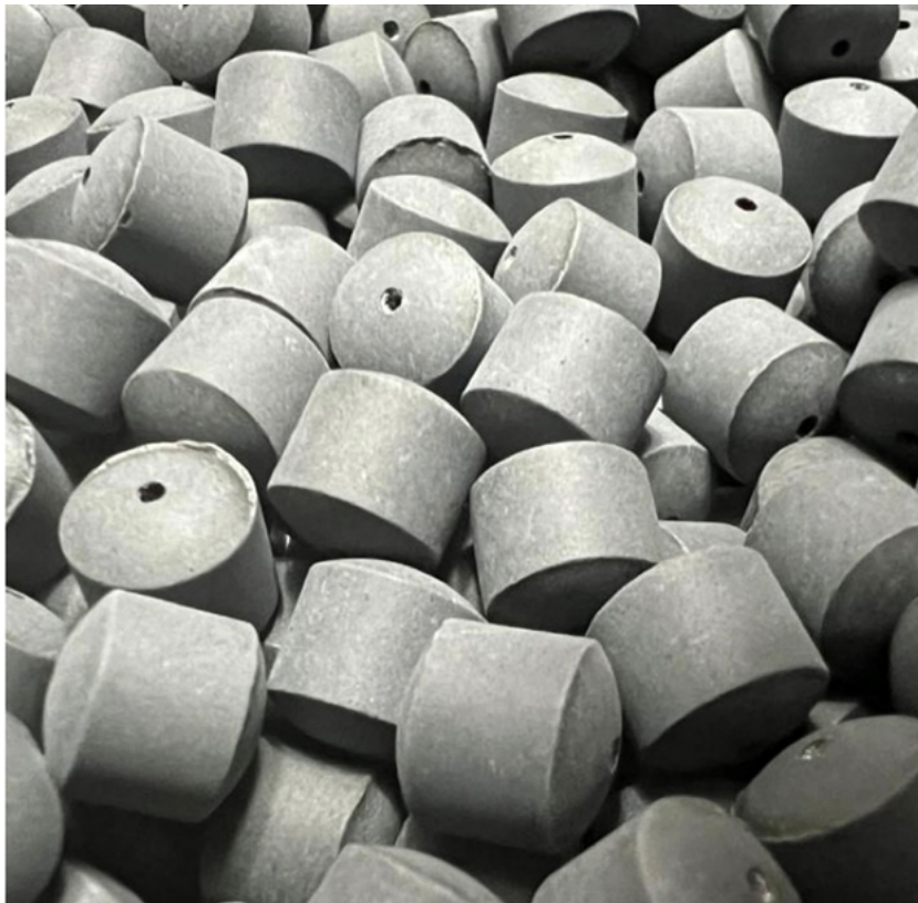
Figure 1: Cylindrical-shaped pellets obtained from the processing of volcanic rock material and marketed as Kiko Technology. The water-insoluble pellets weigh 0.8gm and measure 8x8mm with a 1mm central hole.
