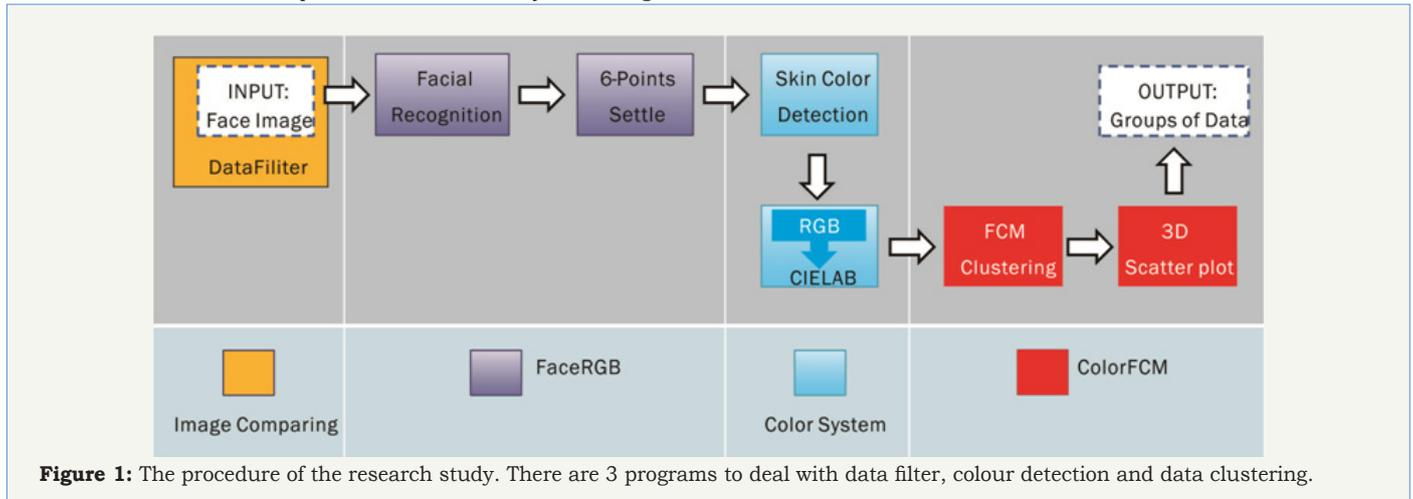
**Figure 1:** The procedure of the research study. There are 3 programs to deal with data filter, colour detection and data clustering.
