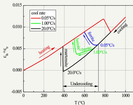
**Figure 1:** Illustration of internal stress evolution during heating/cooling.
