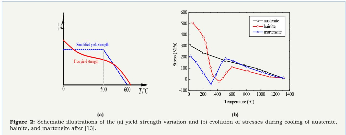
**Figure 2:** Schematic illustrations of the (a) yield strength variation and (b) evolution of stresses during cooling of austenite, bainite, and martensite after [13].
