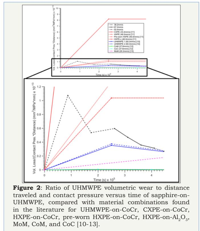
**Figure 2:** Ratio of UHMWPE volumetric wear to distance traveled and contact pressure versus time of sapphire-on-UHMWPE, compared with material combinations found in the literature for UHMWPE-on-CoCr, CXPE-on-CoCr, HXPE-on-CoCr, pre-worn HXPE-on-CoCr, HXPE-on-Al<sub>2</sub>O<sub>3</sub>, MoM, CoM, and CoC [10-13].
