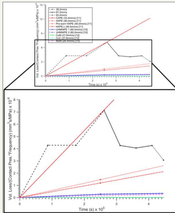
**Figure 3:** Ratio of UHMWPE volumetric wear to frequency and contact pressure versus time of sapphire-on-UHMWPE, compared with material combinations found in the literature for UHMWPE-on-CoCr, CXPE-on-CoCr, HXPE-on-CoCr, pre-worn HXPE-on-CoCr, HXPE-on- $\text{Al}_2\text{O}_3$ , MoM, CoM, and CoC [10-13].
