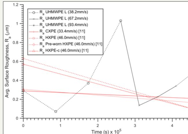
**Figure 5:** Comparative UHMWPE surface roughness versus time of sapphire-on-UHMWPE experiments and of surface roughness data of CXPE-on-CoCr, HXPE-on-CoCr, pre-worn HXPE-on-CoCr, and HXPE-on-Al<sub>2</sub>O<sub>3</sub> [11].
