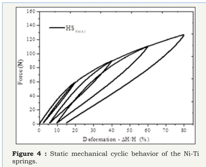
Figure 4 : Static mechanical cyclic behavior of the Ni-Ti springs.
