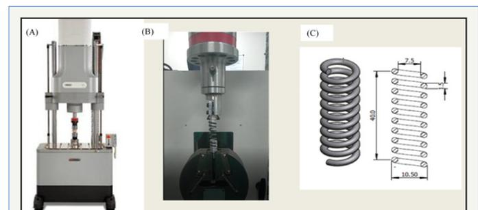
**Figure 2 :** Mechanical tests of the Ni-Ti SMA springs. (A) Electro Pulse E10000 Dynamic Machine. (B) Experimental Assembly for test. (C) Mechanical design and dimensions in mm of the Ni-Ti SMA helical springs: height (H) - 40, inner diameter (Di) - 7.5, outer diameter (De) - 10.5, wire diameter (d) - 1.5.
