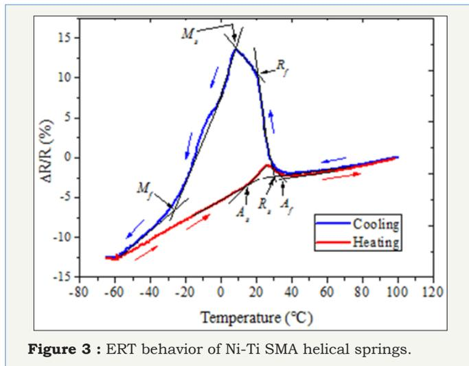
Figure 3 : ERT behavior of Ni-Ti SMA helical springs.
