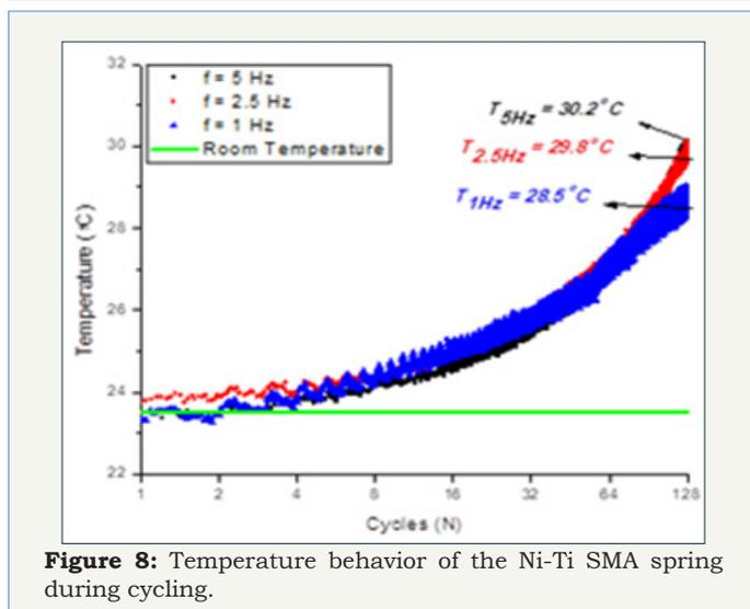
**Figure 8**: Temperature behavior of the Ni-Ti SMA spring during cycling.
