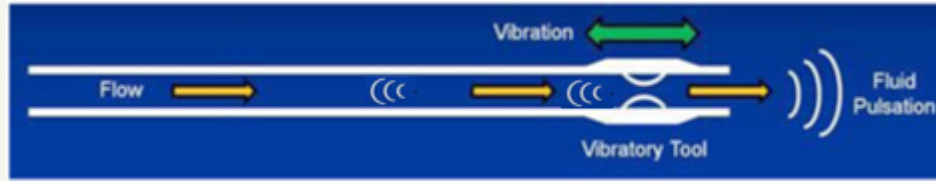
Figure 1: Working mechanism of hydraulic axial vibratory tool [22].
