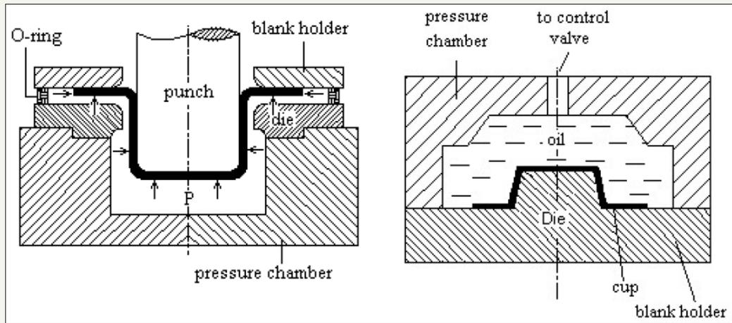
Figure 1: Schematic diagram of sheet hydroforming: (a) sheet hydroforming-punch, (b) sheet hydroforming-die.
