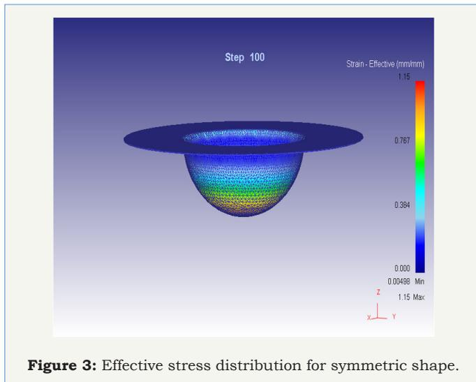
**Figure 3:** Effective stress distribution for symmetric shape.
