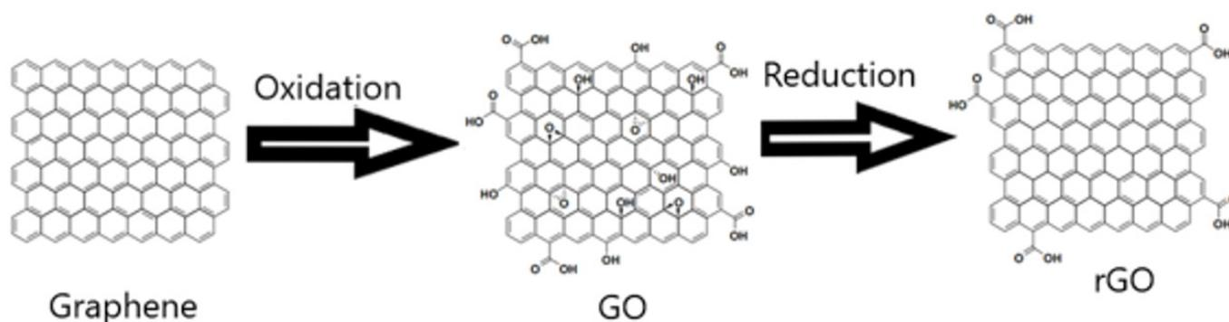
**Figure 2:** Schematic representation of structures of graphene, GO and rGO.
