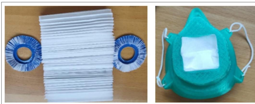
**Figure 7:** Placement of the HEPA filter in the Lowells Makes mask printed in PLA cut from a coil.
