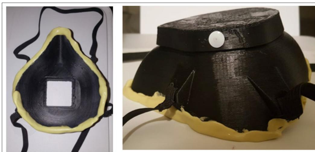
**Figure 8:** Additional fixing of the cover using office tacks and addition of a heavy silicone flexible seal to the Lowells Makes mask printed in PLA.
