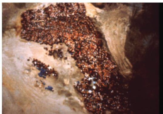
Figure 2: Is an aerial photograph of a drum disposal site. The photo allows counting and documenting the number of containers and changes over time.
