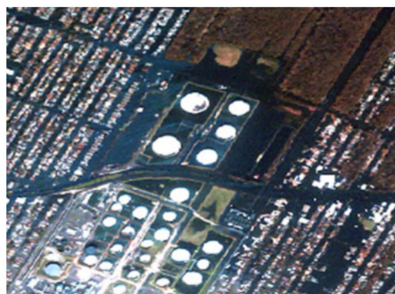
Figure 4: Oil spill from failed containment of a storage facility during Hurricane Katrina. The spill is represented by a light blue sheen on the water. Source: The EPA/Environmental Photographic Interpretation Center (EPIC).
