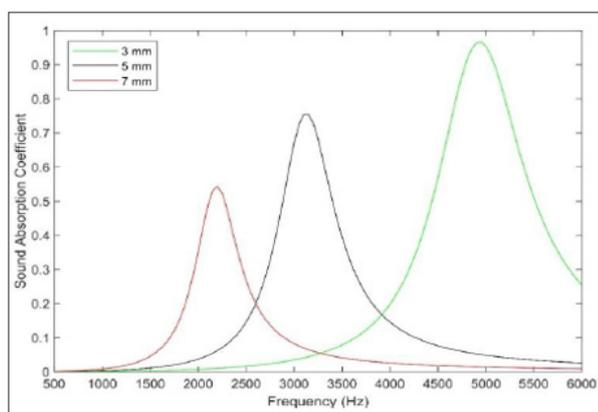
**Figure 4:** Effect of varying distance between the perforations on SAC of the MPP.
