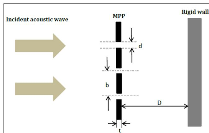
**Figure 1:** Schematic diagram of MPP.
