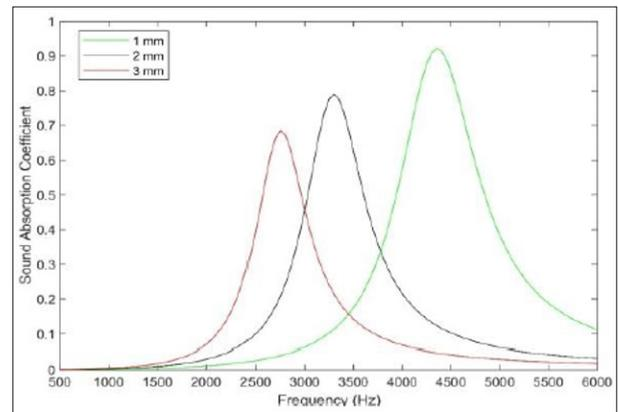
**Figure 2:** Effect of varying thickness on SAC of the MPP.
