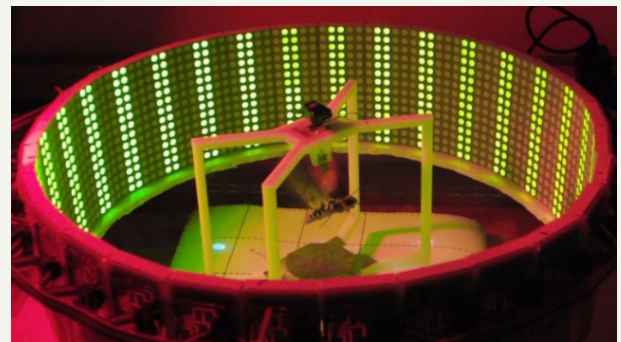
Figure 5: Scientists have created novel method for electronically manipulating the flight muscles of moths and monitoring the electrical signals moths use to control those muscles. Image Credit: Alper Bozkurt [12].
