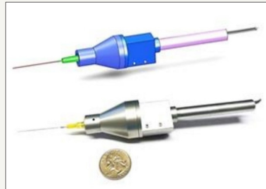
Figure 4: The CAD model and prototype of the fiber-optic-sensor-based microsurgical tool, SMART. Image Credit: Courtesy Cheol Song, Johns Hopkins University [10].
