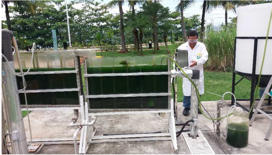
Figure 2: Closed system to obtain micro-algal biomass running at Petrobras R&D Center.
