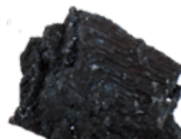
Figure 4: Pseudomorph hematite after magnetite.
