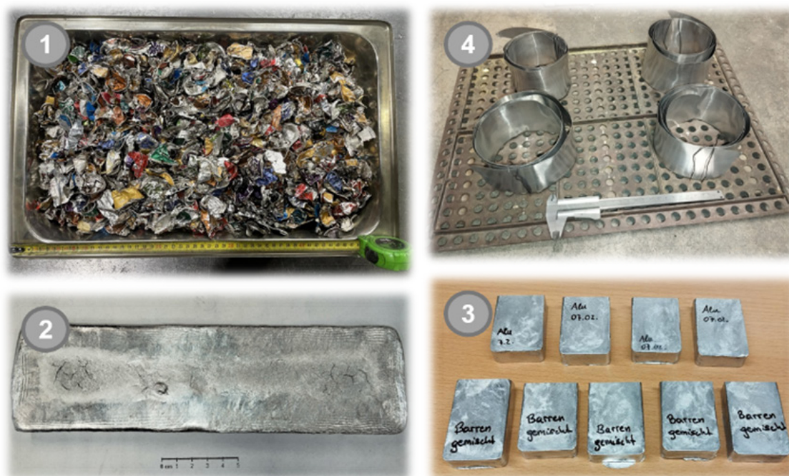
Figure 2: Representation of (1) Pre-processed capsules, (2) Aluminium ingot after remelting by adding a salt mixture, (3) Smaller ingots after cutting and remelting, (4) Produced aluminium sheets.
