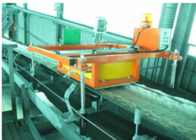
Figure 14: Online XRF analyzer measuring iron (Fe) and titanium (Ti) concentration in dry and wet feldspar.
