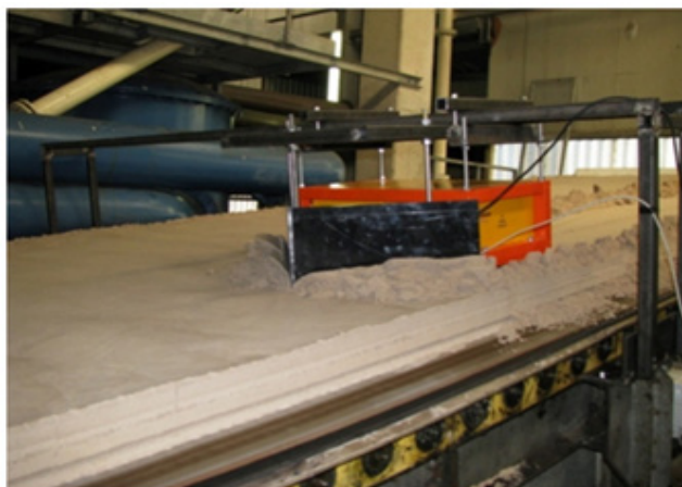
Figure 11: Online XRF analyzer measuring aluminum (Al) and iron (Fe) concentration in quartz sand.
