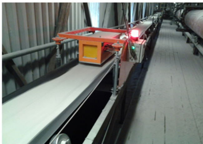
Figure 2: Online XRF analyzer measuring iron (Fe) concentration in nepheline syenite.
