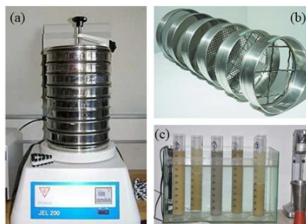
Figure 5: a) Vibrating sieves. b) Sieves with square mesh of various and decreasing sizes. c) Sedimentation apparatus.
