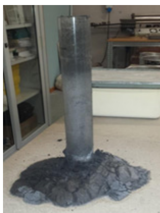
Figure 6: reaction between Al dust and \text{H}_2\text{O} during sedimentation test.
