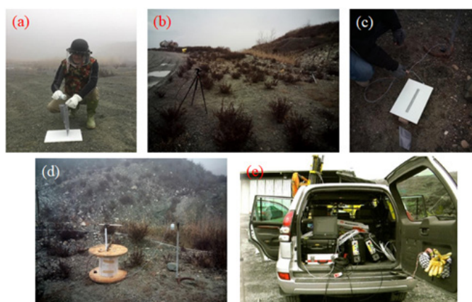
Figure 21: a) Kevlar helmet and bib. b) AOS camera. c) “Template” for placing the dust. d) Air blast sensor (1 meter from the “dark shot”). e) Mobile instrument acquisition centre.
