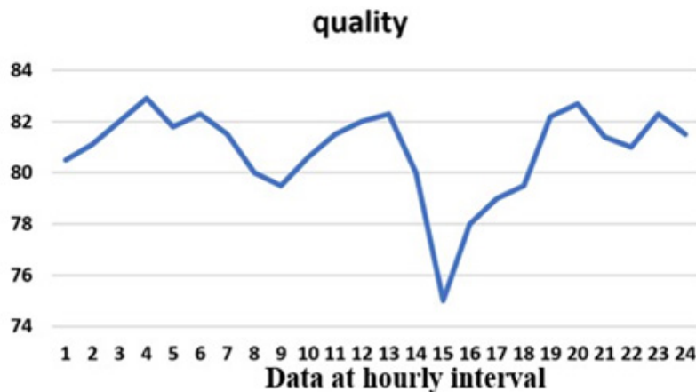
Figure 4: Change in quality of sponge iron product as a function of time (time step is one hour).
