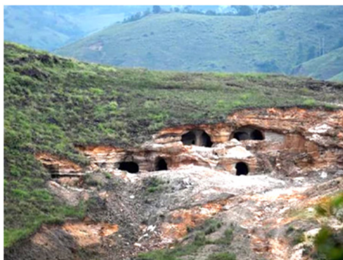
Figure 1: Rat-hole mine in Sutunga area.
