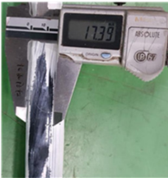
Figure 5: Decontaminated area by the circular nozzle.
