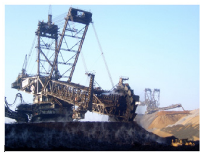
Figure 1: Bucket wheel excavator in Hambach mine extracting lignite in a deep cut.
