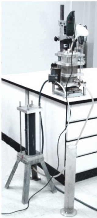
Figure 2: Laboratory equipment for grouting sand columns [10-13].
