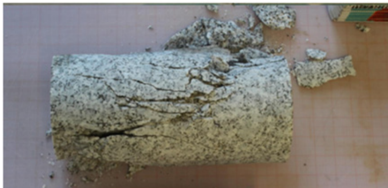
Figure 12: Uniaxial compression failure of granite. From [15].
