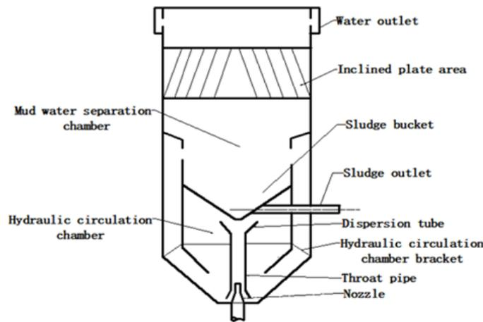
Figure 1: Schematic diagram of deep clarification device.
