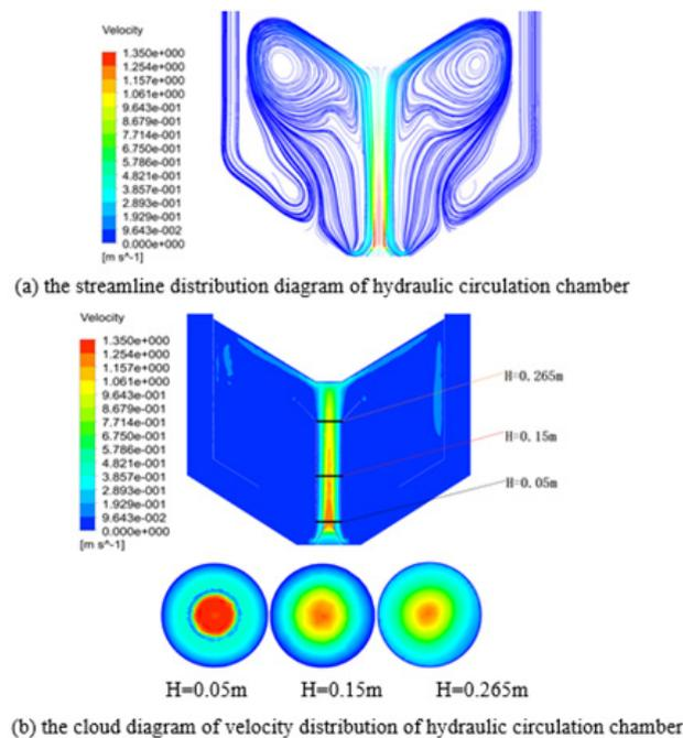
Figure 2: The CFD numerical simulation of hydraulic circulation chamber.
