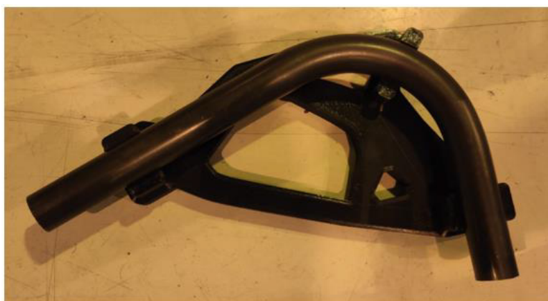
Figure 5: Manufactured check form tool and the steel tube.
