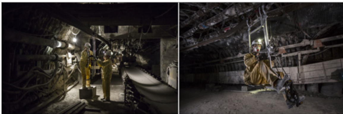
Figure 1: A view of the new miners' bike during the underground tests.
