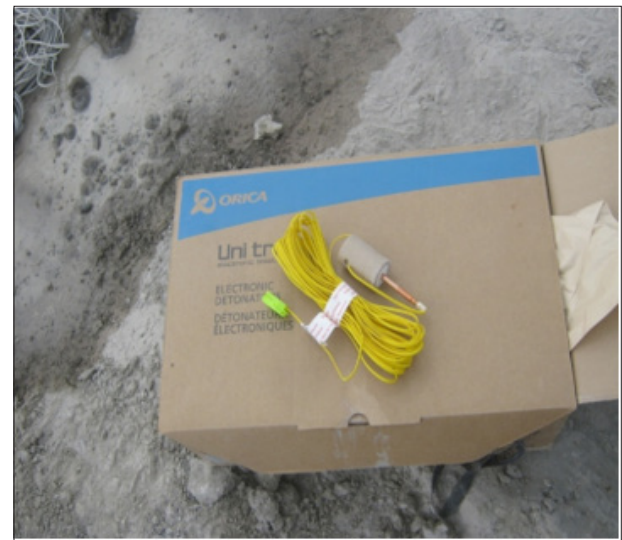
Figure 10: Electronic delay detonator.
