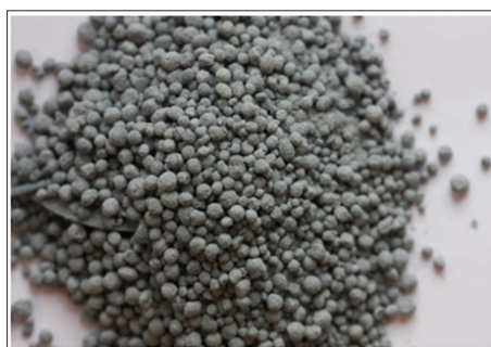
Figure 2: Raw materials: 1-4mm pellets made of \text{SiO}_2 and SiC.
