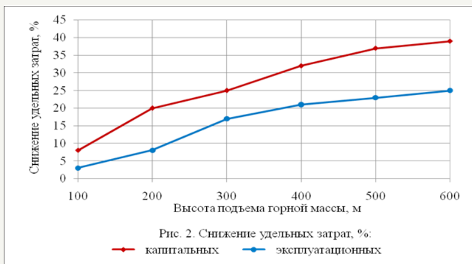
Figure 1: Change of specific capital and operating costs for crushing and conveyor complexes depending on the hoisting height of the rock mass and the angle of inclination of the conveyor elevator: inclination angle of the conveyor ( \beta ), height of material hoisting ( h_n ), specific capital ( K_{уд} ) and operating ( \mathcal{E}_{уд} ) costs.
