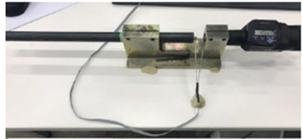
Figure 4: Digital micrometer and calibration set-up.
