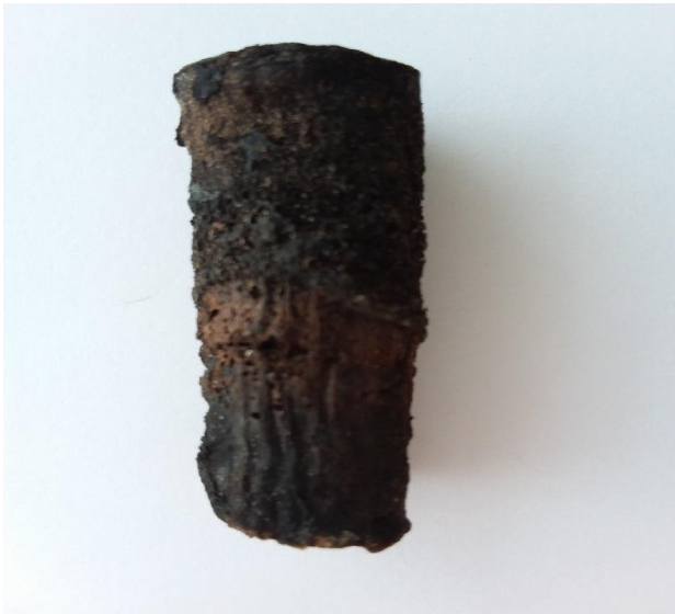
Figure 11: This cork has a charred appearance.
